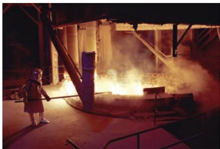
A furnace operator takes a sample before pouring the liquid aluminum oxide.
