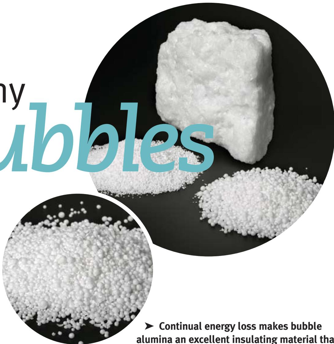
► **Continual energy loss makes bubble alumina an excellent insulating material that can withstand exceptionally high temperatures.**
